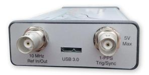
1. 10 MHz Reference input / output. Use a clean 10 MHz reference sine wave or square wave with >0 dBm level. A +13 dBm sine wave input or 3.3V CMOS clock input is recommended.
